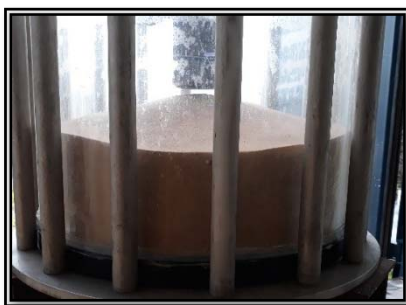
Figures 5 & 6: Before and after images of testing of the fluidisation nozzle.
