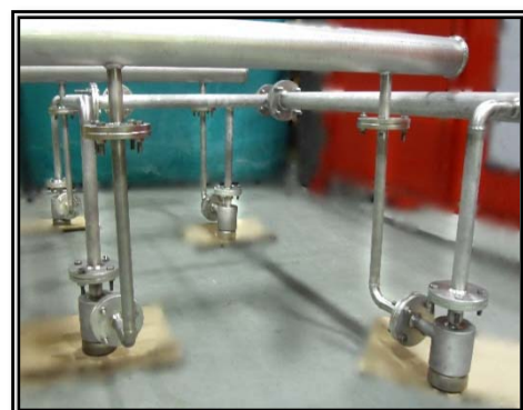
Figures 11 & 12: 8 nozzles, arranged as 2 banks of 4, to prevent solids deposition across a 4-cell Induced Gas Flotation Vessel. The internals were designed and built as a retrofit to be installed between existing equipment.
