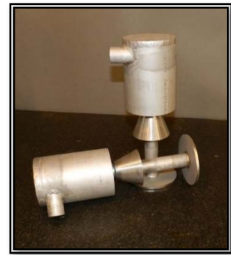
Figure 3: Localised jetting nozzle installed above vessel drain points.
