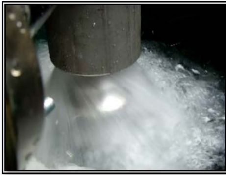
Figure 7: Early testing of the cyclonic effect on the zone of influence.
